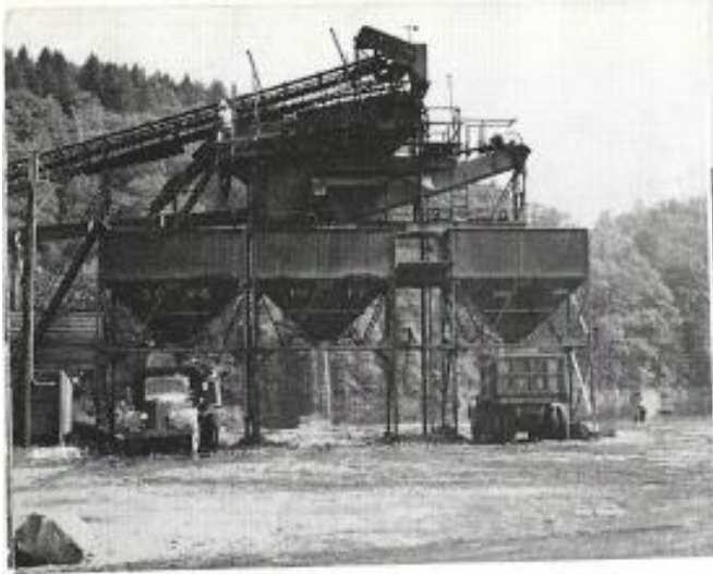
Trucks pick up sand or segregated gravel from bins at the processing plant.
