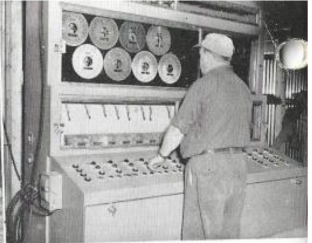
Operator of the concrete mixing plant sets the mix from this control panel.
